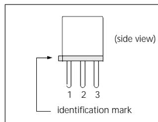
Fig 1c. Pin Layout
