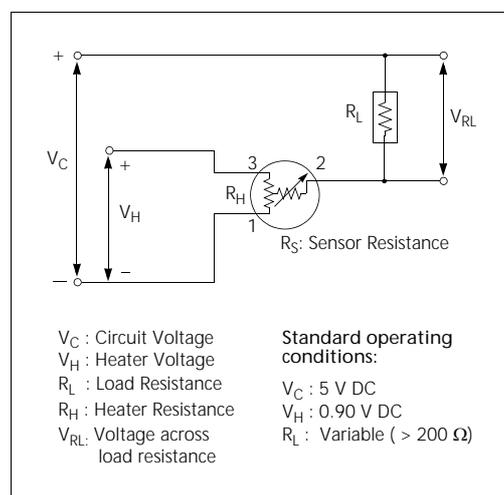
Fig 2. Standard circuit
