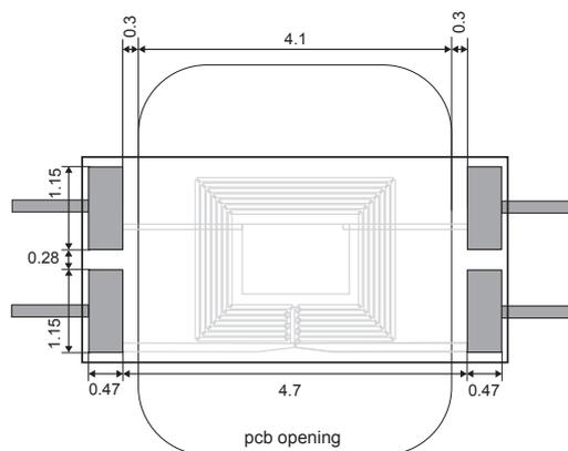
For shortest response time, in case of mounting onto a printed circuit board (PCB), HMC03M shall be positioned over an opening to allow enough air circulation around the sensor.
