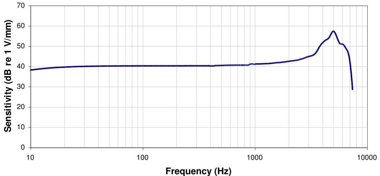
The above plot shows a typical frequency response curve for a device clamped below and subjected to piston-like displacement to the face of the rubber sensing pad.
