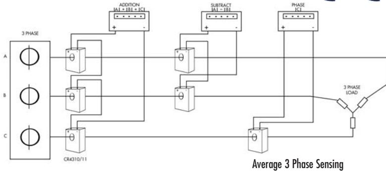
All single phase current transducers are available in split core design. Simply put an "S" at the end of the prefix\*
