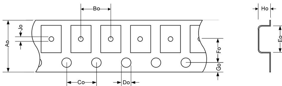
Figure 5: Tape information (drawing not to scale)
