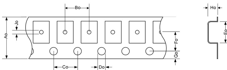
Figure 5: Tape information (drawing not to scale)
