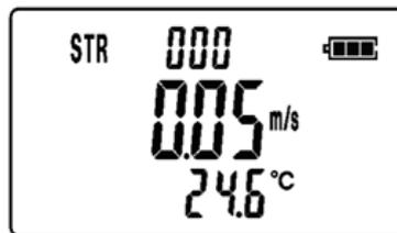
Hold the reading by pressing the **ENTER HOLD** key.
