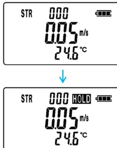
While measuring, press the **ENTER/HOLD** key to hold the current reading.
