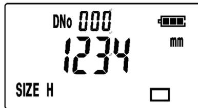
Set the height (H) with **▲** **▼** keys and press the **ENTER HOLD** key.
