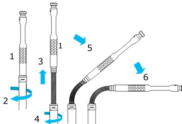
1. Hold the upper part 1 of the probe, and unscrew 2.
