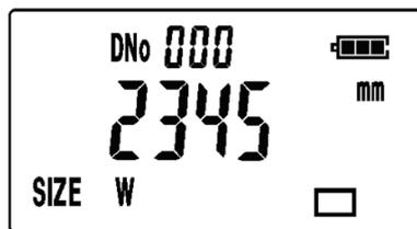
Set the width (W) with **▲** **▼** keys and press the **ENTER HOLD** key.
