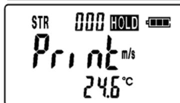
When printing is complete, the screen will return to the measurement screen with the reading held. Measurement can be resumed by releasing the hold mode.
