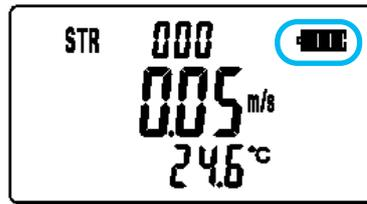
Check the "Battery Level Indicator" to confirm the remaining battery level. The battery consumption rate largely depends on the measured air velocity. When the batteries need to be replaced (or recharged), the indicator will start blinking.
