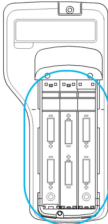
4. Insert the batteries according to the indicated polarity chart. The instrument requires six (6) AA size batteries. Types of batteries that can be used are: Manganese, Alkaline, Ni-Cd batteries, or Ni-MH batteries. The six (6) batteries must be of the same type. DO NOT mix different types of batteries. Failure to observe this may cause battery leakage or damage to the instrument.
