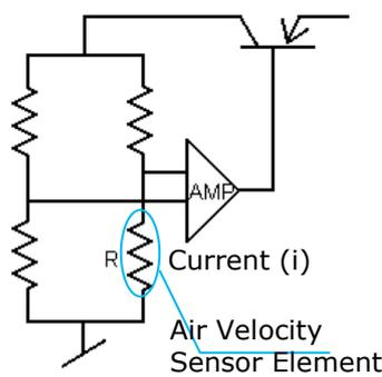
The *Anemomaster* anemometer is based on the above principle. Generally, a hot-wire anemometer employs a feedback circuit to control the sensor to maintain constant temperature. (Constant Temperature Type)
