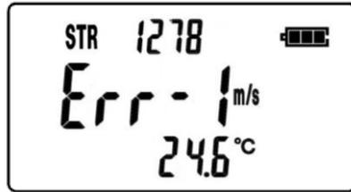
The number of stored data records has exceeded the maximum limit of 1500 data records. Stored data must be deleted to enable further data storage.
