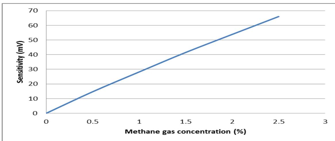
Fig. 2 Linearity to methane gas till 50%LEL
