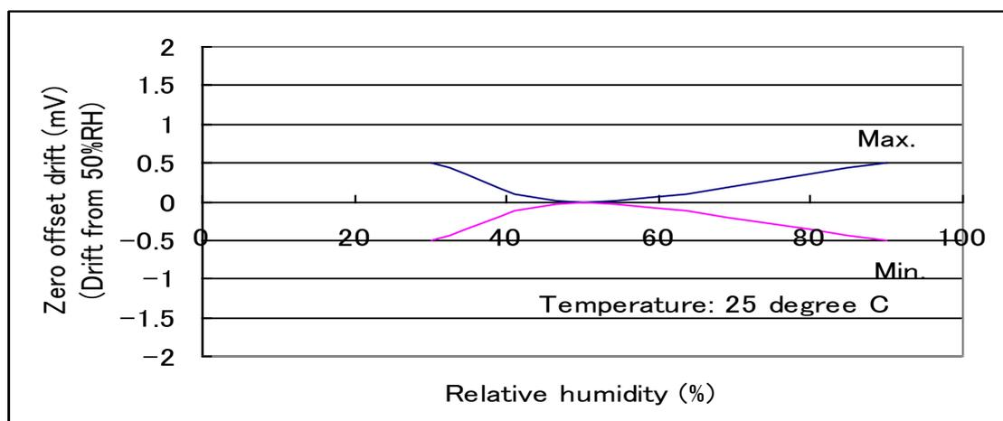
Fig.5 Humidity dependence of zero offset
