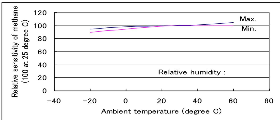
Fig. 4 Temperature dependence of relative sensitivity to methane
