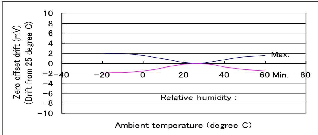
Fig.3 Temperature dependence of zero offset
