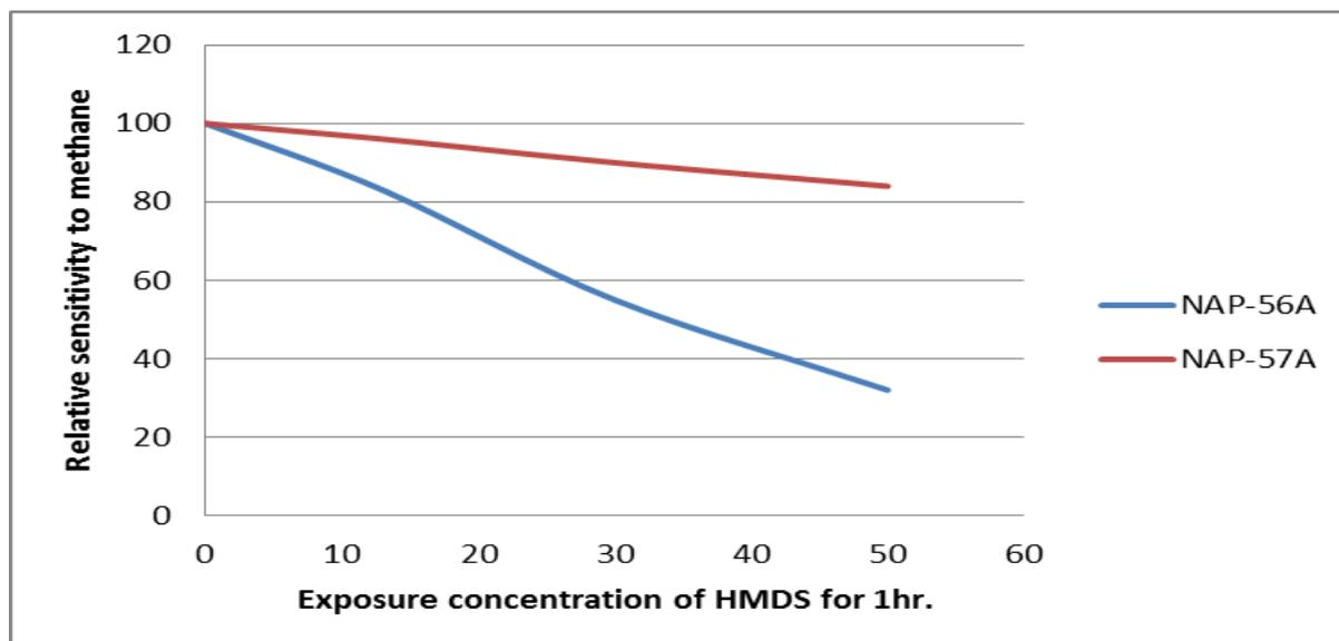
Fig.8. HMDS poisoning resistivity
