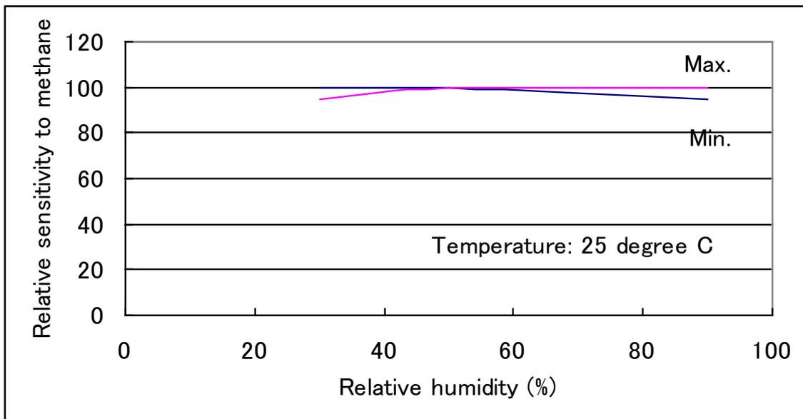
Fig.6 Humidity dependence of relative sensitivity of methane
