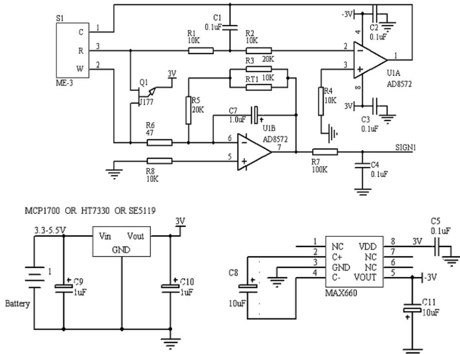
Fig2: ME4-NH<sub>3</sub> test circuit
