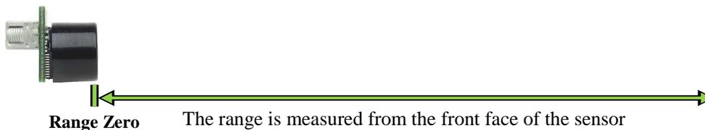
The I2CXL-MaxSonar-EZ will report the range to the closest detectable object. Target detection has been characterized in the sensor beam patterns.
