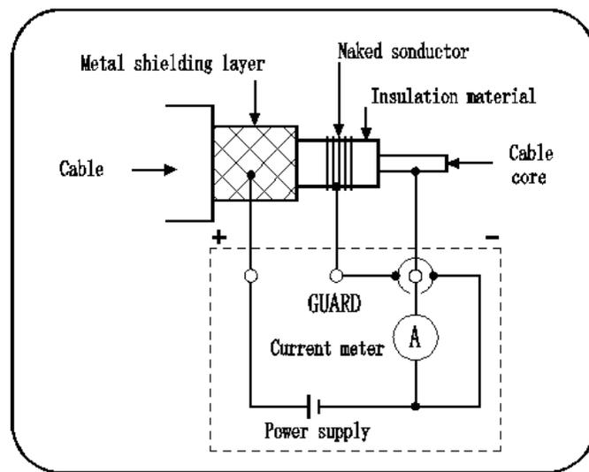
Rc: insulation resistance of the insulation material for high-voltage cables (between core and metal shielding layer)
