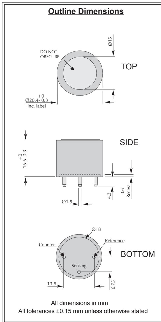
**IMPORTANT NOTE:** Connection should be made via PCB sockets only. Soldering to the pins will seriously damage your sensor.
