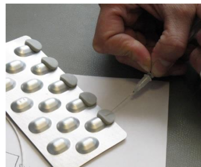
NTH oxygen sensor piercing a blister with septums
