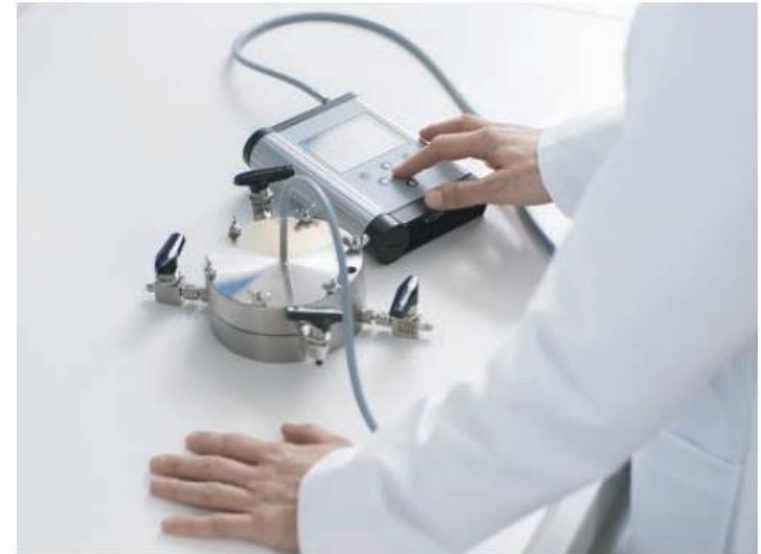
Fig.1: Measurement system set-up: The new measurement cell with two gas connectors for each of the two chambers; the sensor spot is applied to the upper chamber and read out via polymer optical fiber by the Fibox 4 trace.
