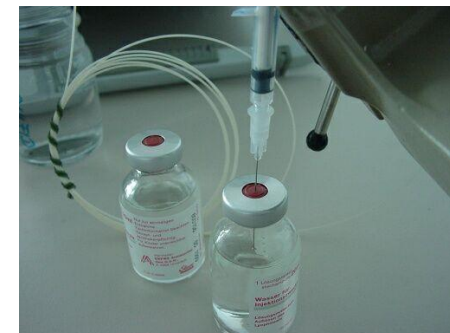
NTH oxygen sensor piercing the septum of a vial
