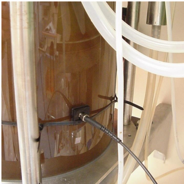
Oxygen sensor integrated inside a 10L bioreactor
