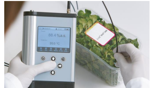
Sensor spots integrated in food packaging
