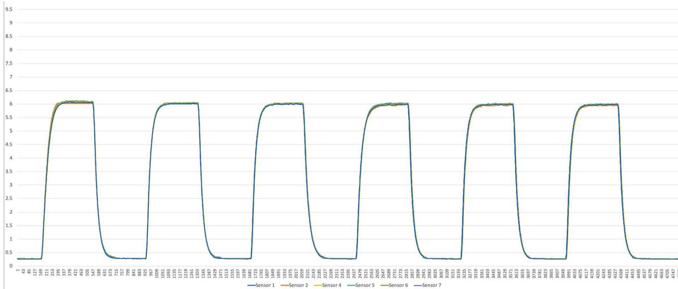
The test results show that the repeatability error range is <math><20\text{ppb}</math> (10ppm  $\pm$  1% of full scale is the normal range);
