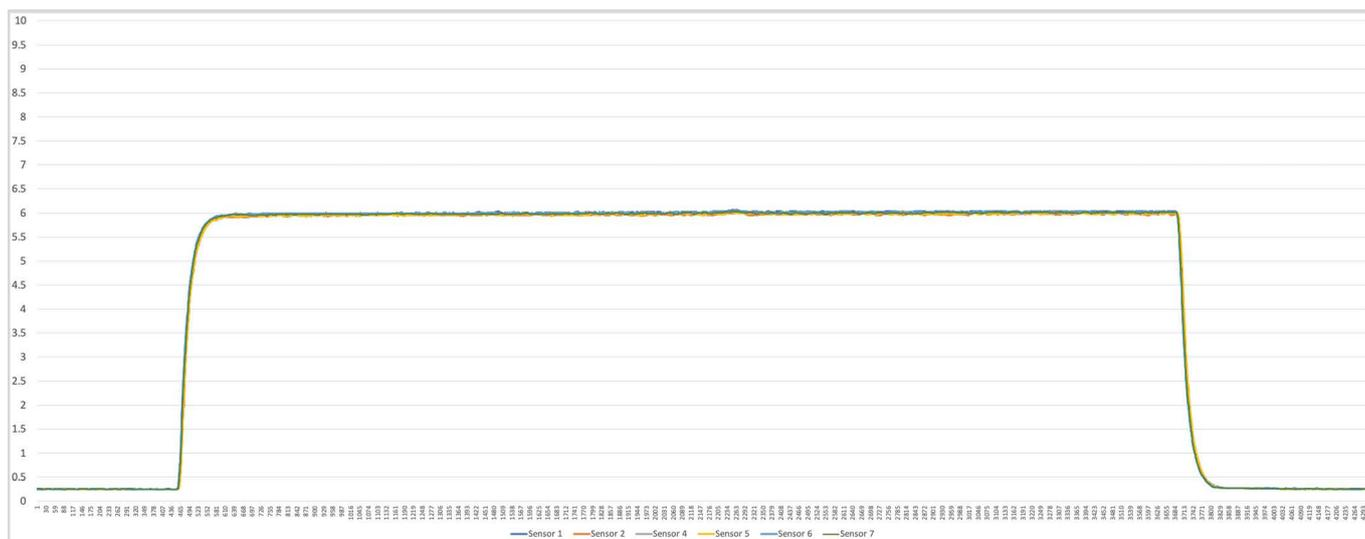
Test result: 2 hours ventilation, range drift <20ppb;
