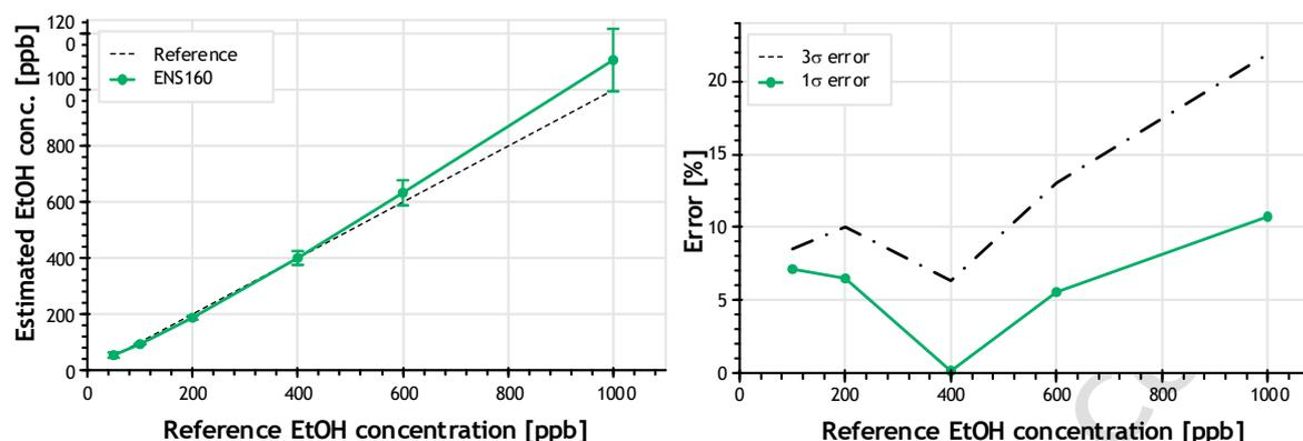
The diagrams show the typical and maximum (3 $\sigma$ ) accuracies of the ethanol signal. A typical error of maximum 10% of the measured value can be derived.
