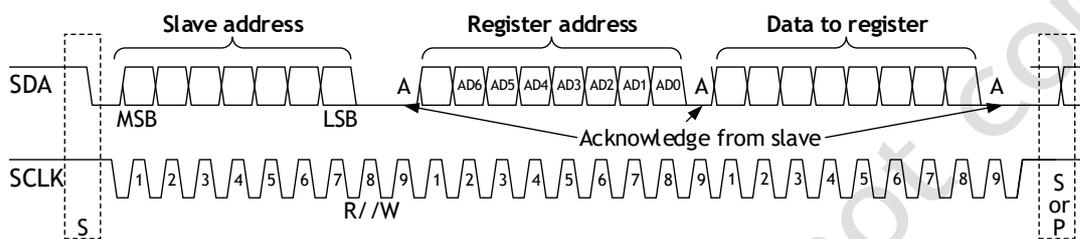
Figure 11: I<sup>2</sup>C Auto-Increment Write Operation
