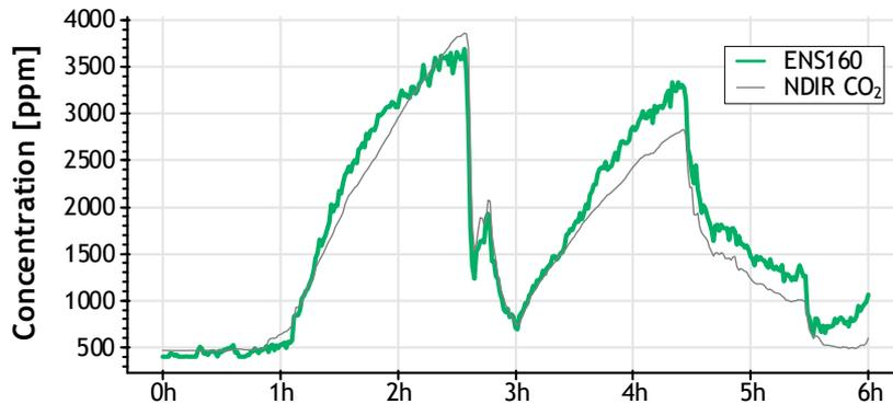
Taking advantage of its RMR<sup>1</sup>-technology, today, the ENS160 reverses the proportional correlation of VOCs and CO<sub>2</sub>, by providing a standardized output signal in ppmCO<sub>2</sub>-equivalents from measured VOCs plus hydrogen, thus adhering to today's CO<sub>2</sub>-standards, as the diagram on the left testifies: ENS160-based equivalent CO<sub>2</sub> estimate vs. CO<sub>2</sub>, detected by an NDIR-sensor during two consecutive meeting sessions, interrupted by a lunch-break.
