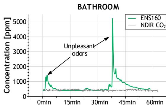
Proven control-algorithms minimize sensor drift and ageing to provide reliable readings over lifetime, thereby making the ENS160's equivalent CO<sub>2</sub> output an affordable solution to truly substitute real CO<sub>2</sub>-based air-quality sensors in the HVAC domain. Please refer to our "Air Quality Solutions" brochure for further information.
