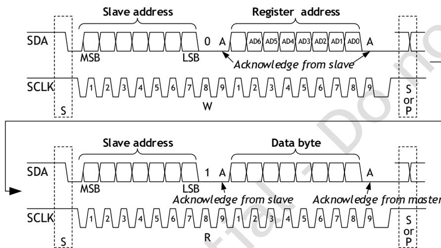
Figure 9: I<sup>2</sup>C Auto-Increment Read Operation
