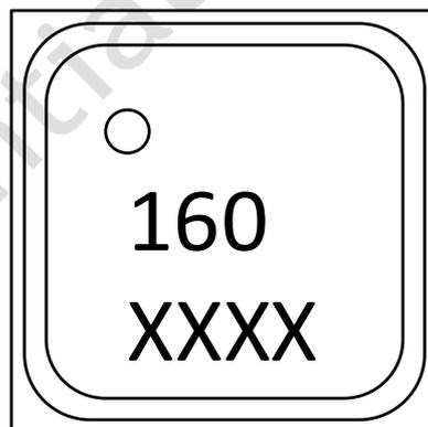
The package has a marking with TC\_4 trace-code according to Cspec 507870020.
