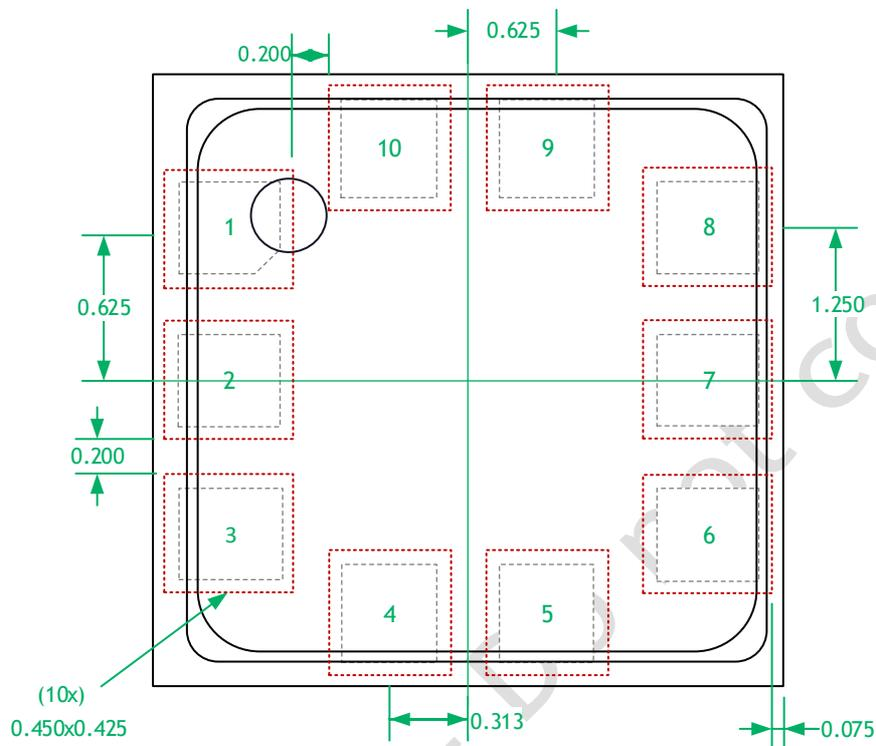
Figure 5 Recommend LGA landing pattern (Top view)
