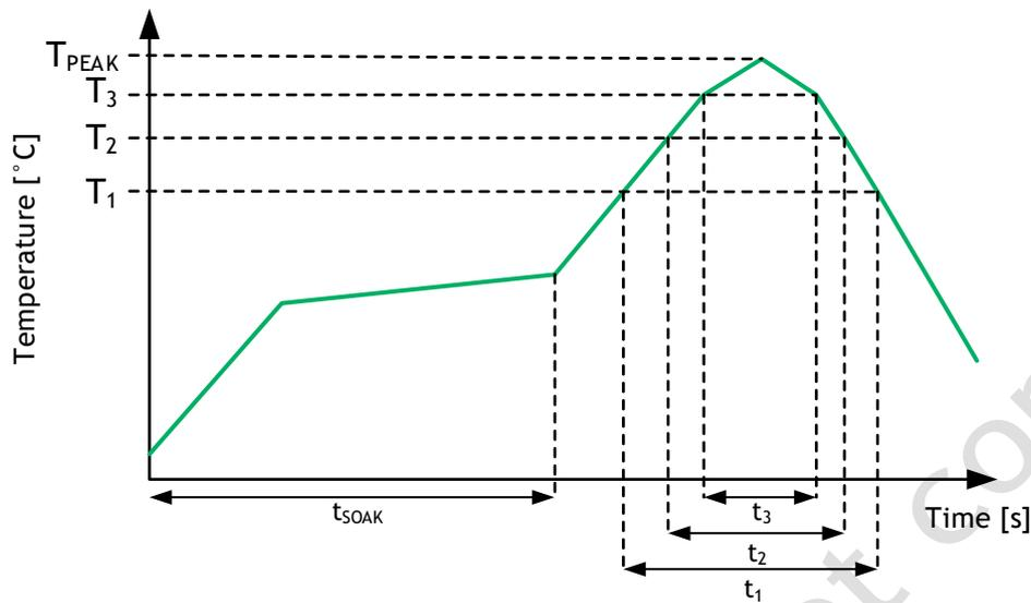
Figure 6 Solder reflow profile graph
