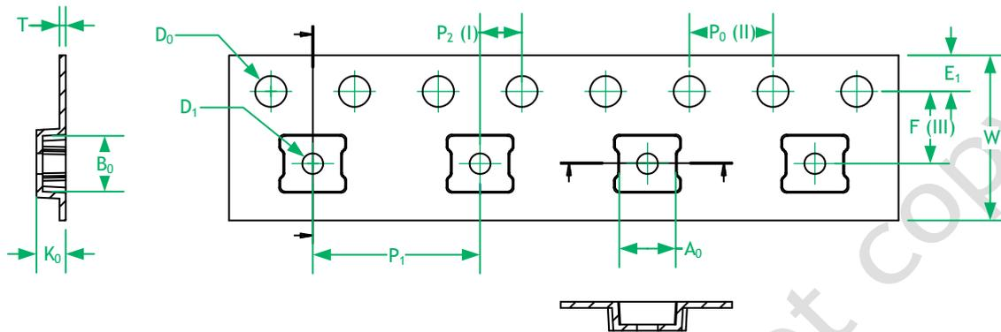
Figure 7 Drawing of the tape & reel
