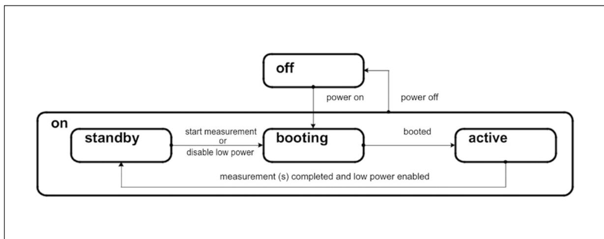
In continuous run mode (see Register [SENS\\_RUN](#)) or when low power is disabled (see Register [SYS\\_CTRL](#)), the device remains in *active* state.
