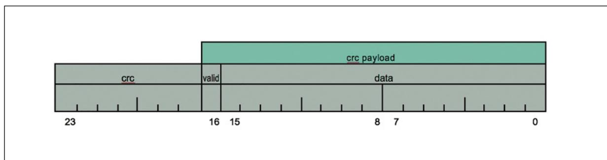
The *checksum* is a cyclic redundancy check over the data and the valid flag; the stored checksum is the result of CRC-7 (polynomial  $x^7+x^3+1$ , see [https://en.wikipedia.org/wiki/Cyclic\\_redundancy\\_check](https://en.wikipedia.org/wiki/Cyclic_redundancy_check)) with 0x7F as initial vector (i.e. with all bits flipped), see [Computing CRC-7](#) for sample C code.
