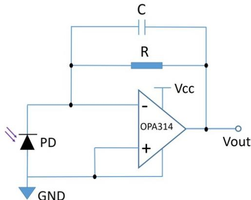
$$V_{out} (V) = I_{ph} (A) \times R (\Omega)$$
