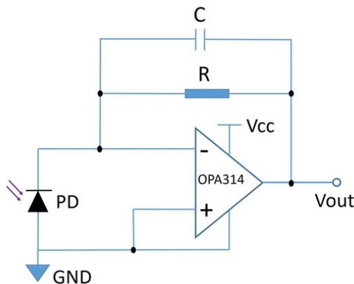
$$V_{out}(V) = I_{ph}(A) \times R(\Omega)$$
