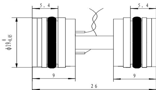
The suggested installation dimension is  $\Phi 19^{+0.05}_{+0.02}$  mm
