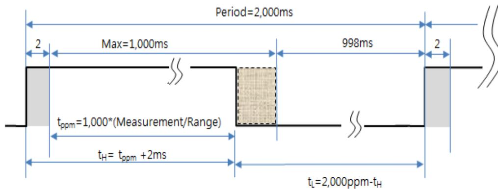
EX)  $t_H$  (High Pulse Width) calculation for 400 ppm in 2,000 ppm Range.
