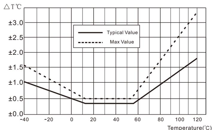
Figure 3 Typical error and maximum error of temperature
