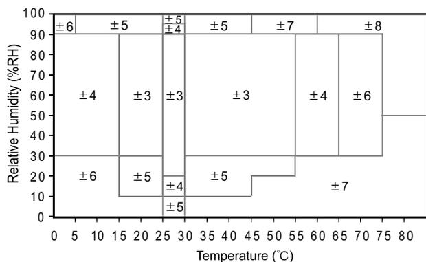
Figure 5 Maximum humidity error between 0~80 °C, unit: (% RH)
