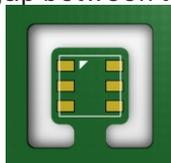
Figure 10 The top view of AHT21 printed circuit board, the design of the milling slit is added in the figure, The heat transfer can be reduced to a minimum.
