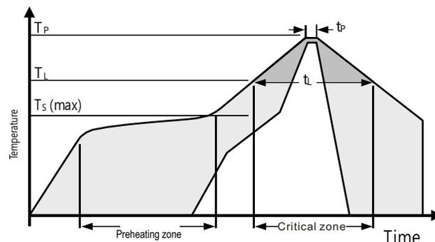
Figure 9 JEDEC Standard welding procedure diagram.  $T_p \leq 260^\circ\text{C}$ ,  $t_p < 30$  sec, lead-free welding.  $T_L < 220^\circ\text{C}$ ,  $t_L < 150$  sec, The rate of temperature rise and fall during welding shall be  $< 5^\circ\text{C}/\text{sec}$ .
