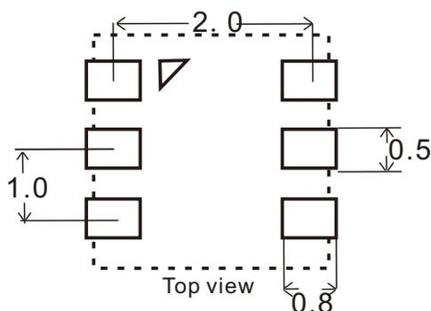
Figure 8 Recommended sensor PCB design size (unit: mm), the outer dotted line is the external size of the SMD package.
