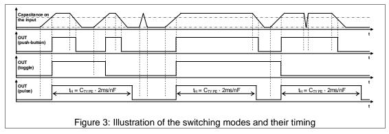
Figure 3 illustrates the switching behaviour for the three modes. Additionally the graph illustrates, that short term disturbances on the sensor are suppressed by the circuit.
