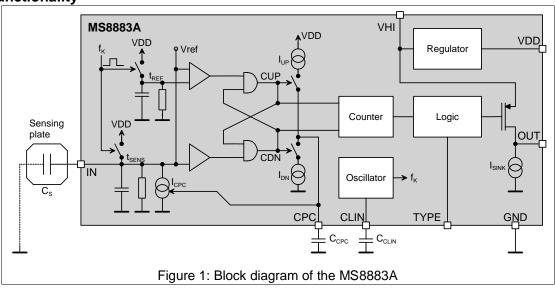
Figure 1 illustrates the functional principle of of the MS8883A.
