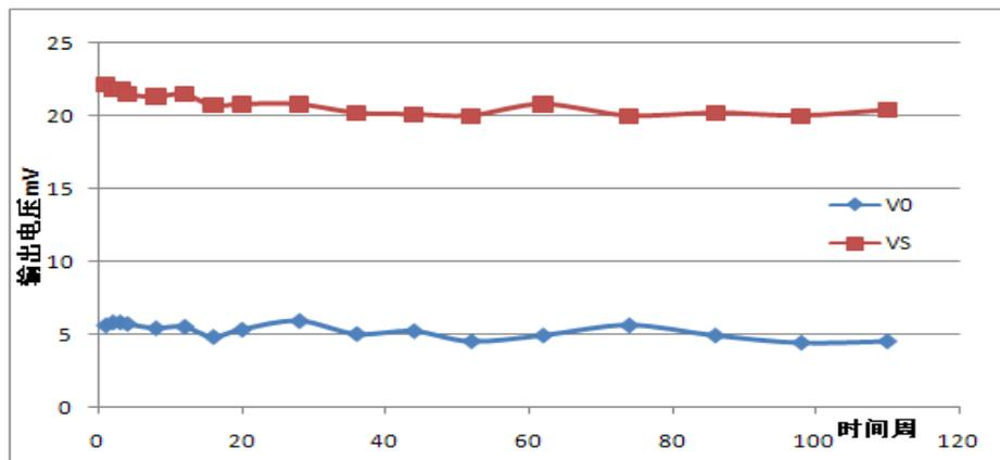
The absolute value of the drift in air is less than 2 mV per year, in 30%CO2 the absolute value of drift is less than 2mV. For a short period storage (in 2 weeks), the sensor need 8 hours preheating to stabilize, for long-term (more than one year) storage, it need more than 48 hours' preheating.
