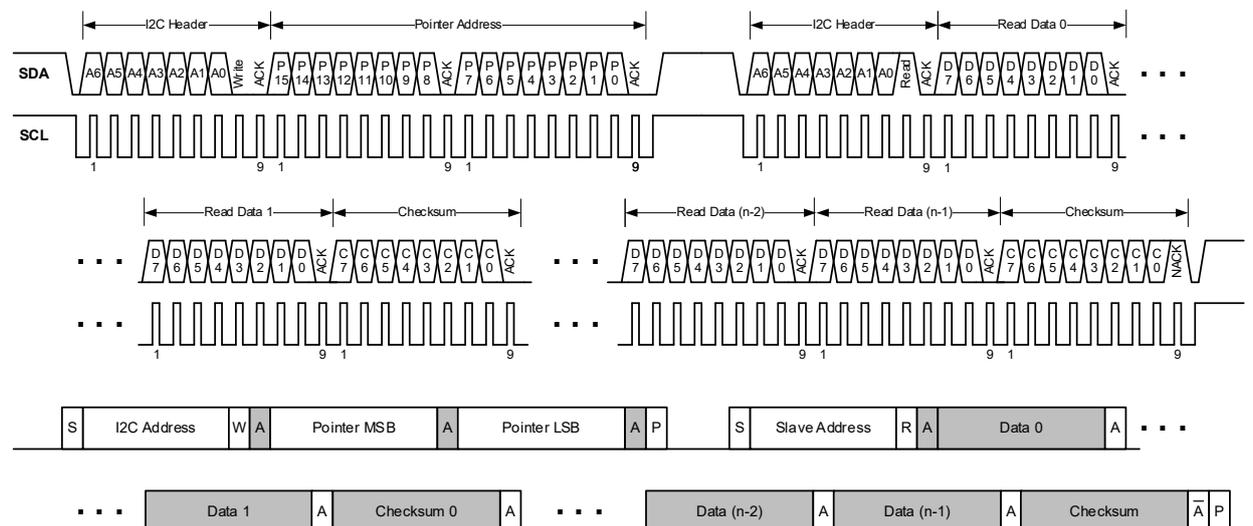
It is allowed to read several times in succession without setting the address pointer again. This reduces the protocol overhead for periodical reading of the measured values.
