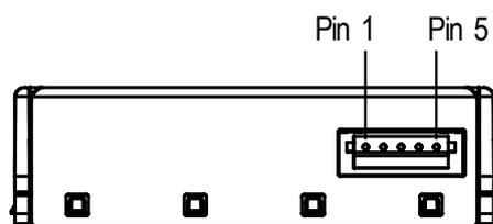
**Figure 1:** The communication interface connector is located at the side of the sensor opposite to the air outlet.
