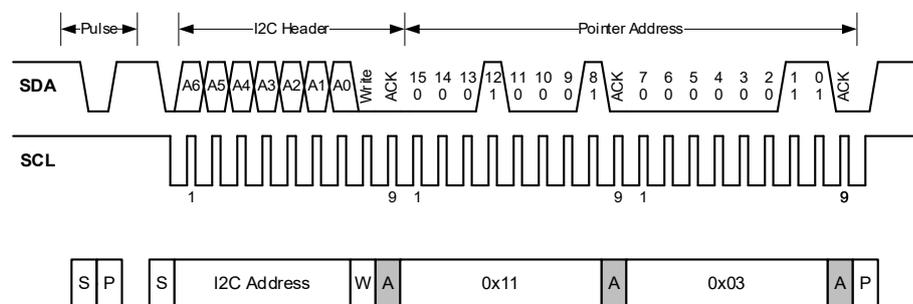
Alternatively, if the software implementation does not allow to send a I2C-Start-Condition followed by a Stop-Condition, the Wake-up command can be sent twice in succession. In this case the first Wake-up command is ignored, but causes the interface to be activated.
