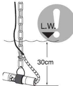
Dispose the sensor in water without air bubbles.
