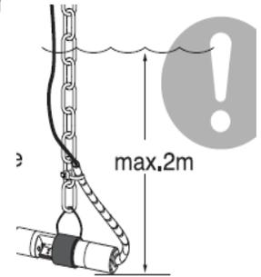
With fluctuation of water level taken into account, dispose the sensor so as to be immersed up to of the order of 30 cm below the expected lowest water level.
