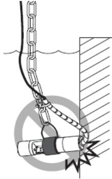
Install the sensor Max.2m below the surface of water.
