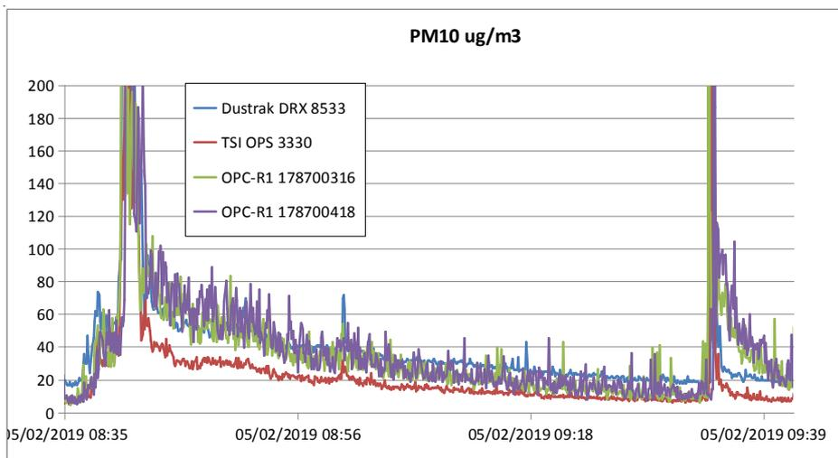
Figure 4 shows a comparison of PM10 monitoring by an OPC-R series sensor and TSI OPS 3330 and DustTrak instruments.
