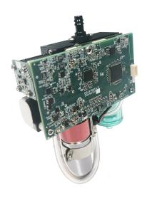
The 9301P-OEM measures up to 30 channels of particle count data from  $0.3~\mu m$  to  $25.0~\mu m$  with a flow rate of 0.1 CFM (2.83 LPM). The assembly is mounted on a plate for ease of integration. The unit includes a particle sensor, particle counter board, integrated vacuum pump and manifold with pre/post filters, real-time clock/calendar with battery backup, logging and data storage for up to 65,000 sample records, communicates via UART and operates from 7-15 VDC.
