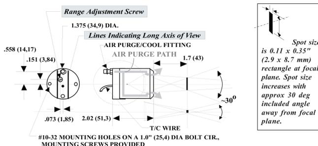
Spot size is 0.11 x 0.35" (2.9 x 8.7 mm) rectangle at focal plane. Spot size increases with approx 30 deg included angle away from focal plane.
