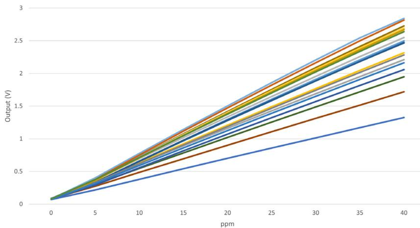
Figure 3 shows the response curve of 20 sensors throughout the entire operating range. Sensors are linear throughout the entire range.
