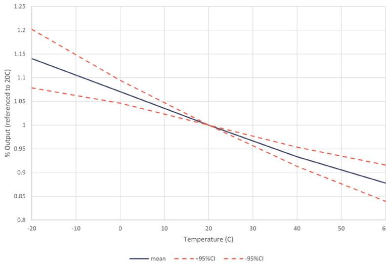
Figure 2 shows the temperature dependence, corrected for the gas law.
