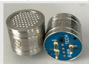
SUSA PID sensor contains the miniature UV lamp, high sensitivity with low noise electronic components and integrated ionization chamber. The standard 4 series compact structure is designed for different application purposes, such as portable, fixed detectors, as well as analyzers. It offers a wide detection range, up to 10000ppm(IBE equivalent) and 5ppb resolution.
