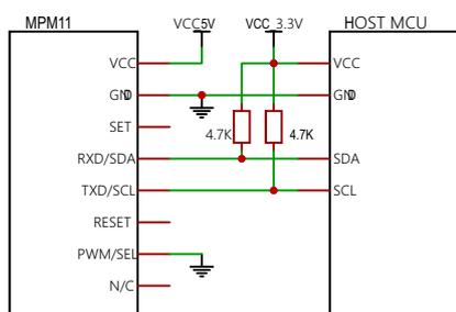
Circuit connection of IIC interface
