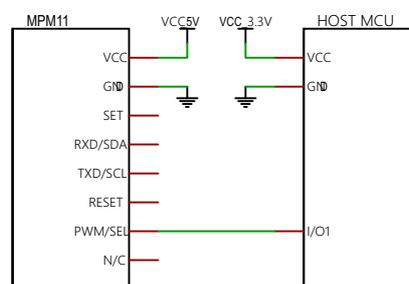
Circuit connection for PWM output
