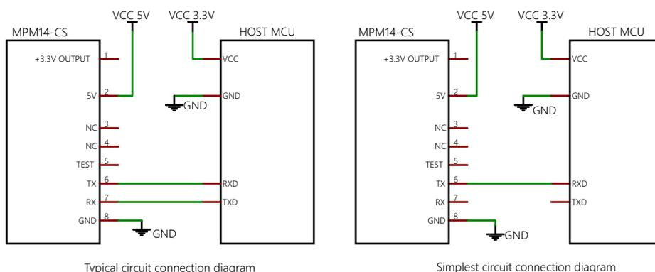
Typical circuit connection diagram
