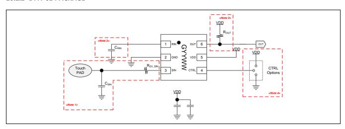
**NOTE:**  $R_{EXT\_SIN} = 200 \Omega$ ,  $C_{SIN} = 1pF$ ,  $C_{RIN} = 1pF$  (recommend)
