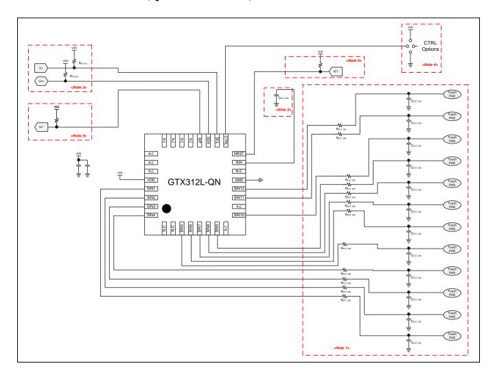
**NOTE:**  $R_{EXT\_SIN} = 560\Omega$  (recommend),  $R_{PU\_I2C} = 10K\Omega$  (recommend)
