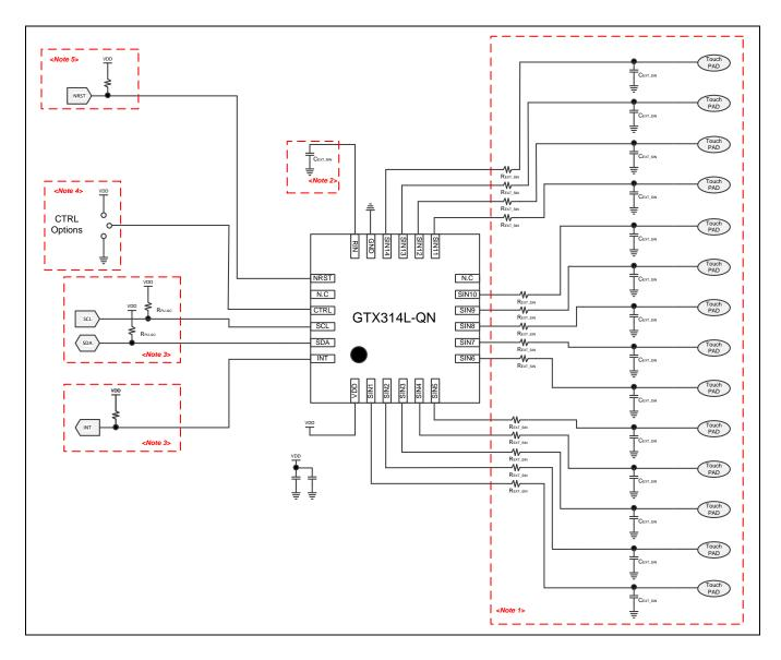
**NOTE:**  $R_{EXT\_SIN} = 560\Omega$  (recommend),  $R_{PU\_I2C} = 10K\Omega$  (recommend)
