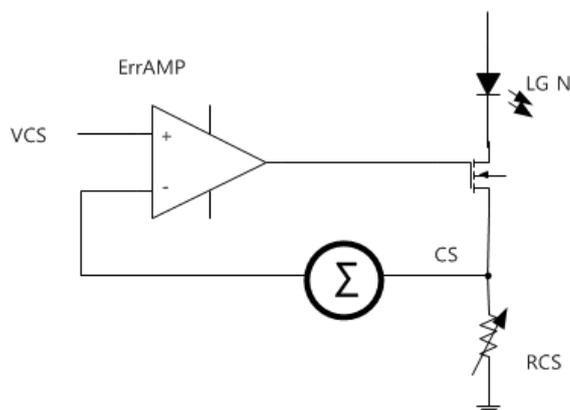
3) When target power is determined, an approximate value of RCS must be chosen by calculating Max.(ILED). One can start with an approximate value of RCS and the final value must be determined experimentally with further fine tuning.
