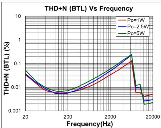
Fig8. THD+N (BTL) vs Frequency
