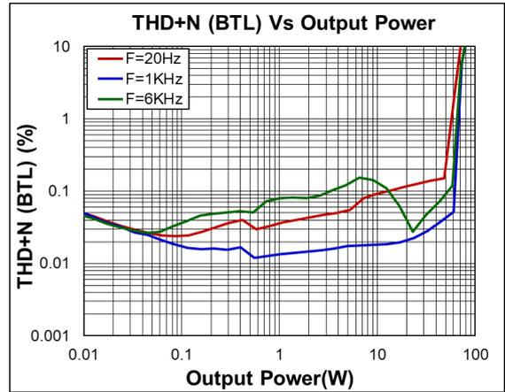
Fig13. THD+N (BTL) vs Output Power
