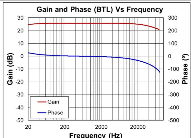
Fig17. Gain and Phase (BTL) vs Frequency
