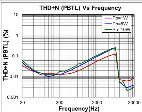
**Fig22. THD+N (PBTL) vs Frequency**
