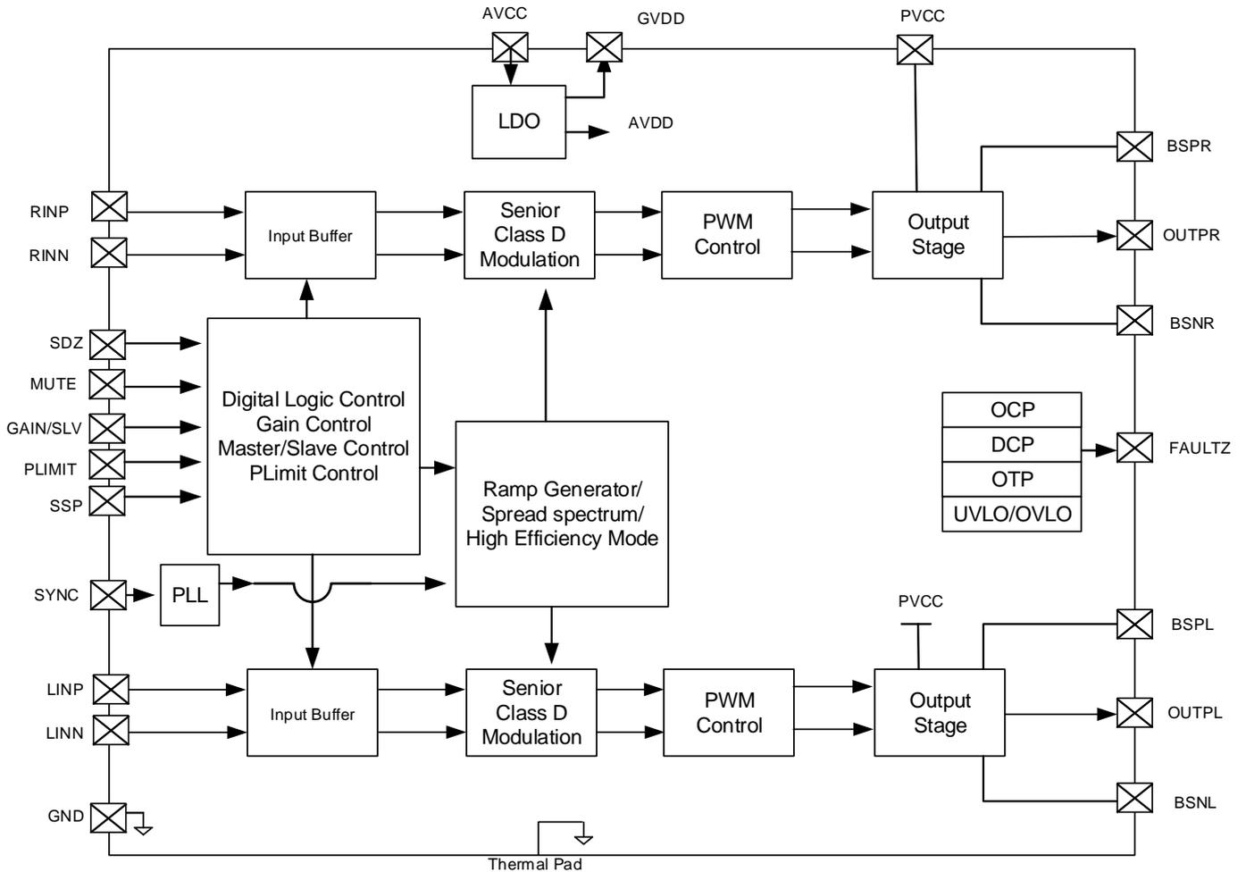
Fig5. iML6603 Functional Block Diagram
