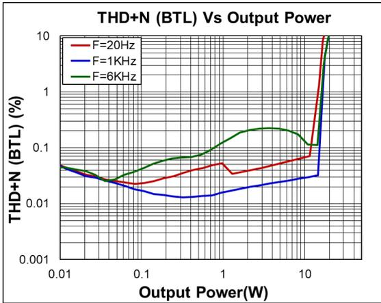
Fig12. THD+N (BTL) vs Output Power
