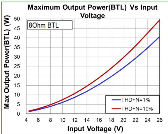
Fig14. Maximum Output Power vs Input Voltage
