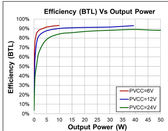
**Fig19. Efficiency (BTL) vs Output Power**
