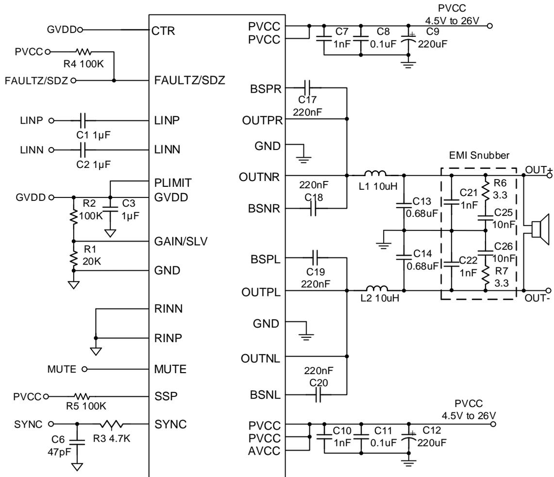
Fig2. Typical PBT Mode Applications
