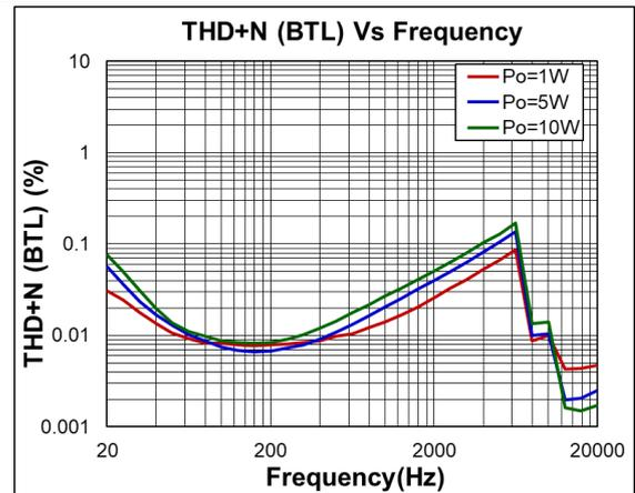
Fig9. THD+N (BTL) vs Frequency
