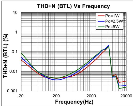
Fig6. THD+N (BTL) vs Frequency
