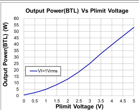
Fig16. Output Power vs Plimit Voltage
