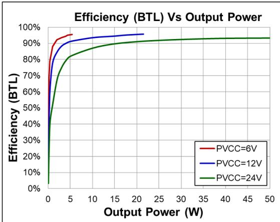
**Fig18. Efficiency (BTL) vs Output Power**
