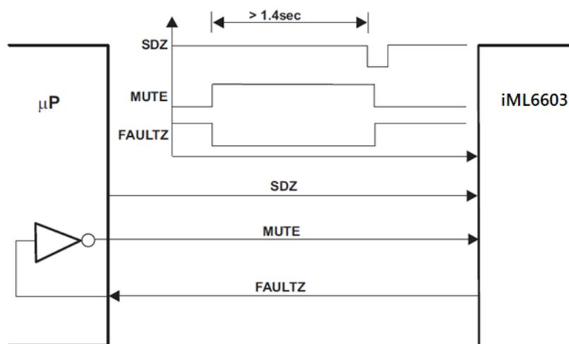
**Fig27. Timing Requirement for SDZ**
