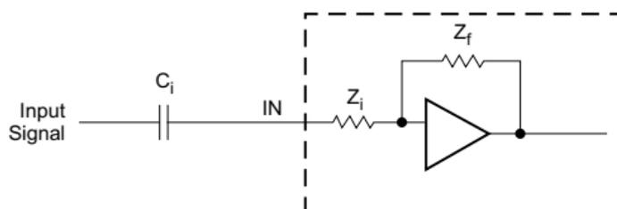
Figure 25. Input Impedance
