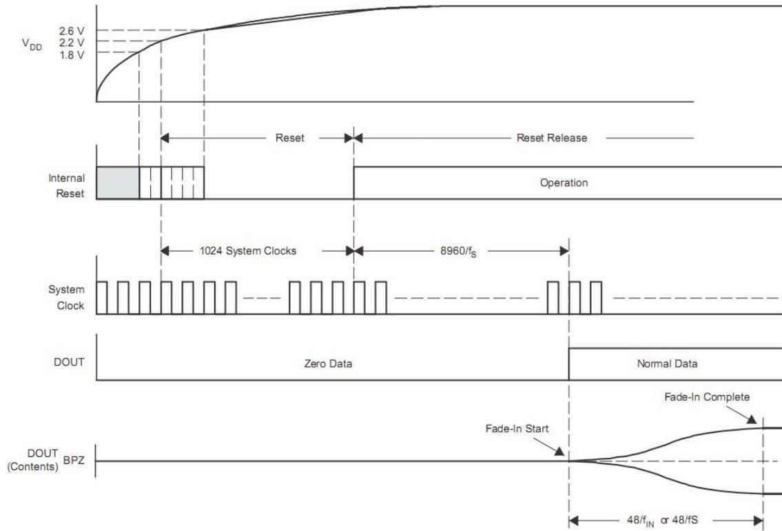
Figure 2. Power-On Timing
