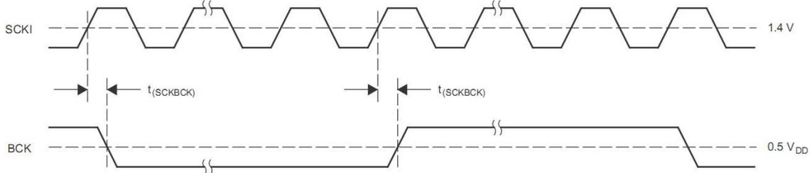
Figure 6. Audio Clock Interface Timing (Master Mode: BCK Works as Output)
