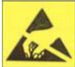
ESD Sensitive Device. This device is manufactured on a CMOS process. It is therefore generically to damage from excessive static voltages. Proper ESD precautions must be taken during handling of this device.
