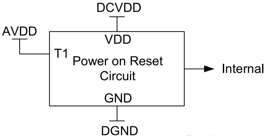
**Figure 6 Internal Power on Reset Circuit Schematic**
