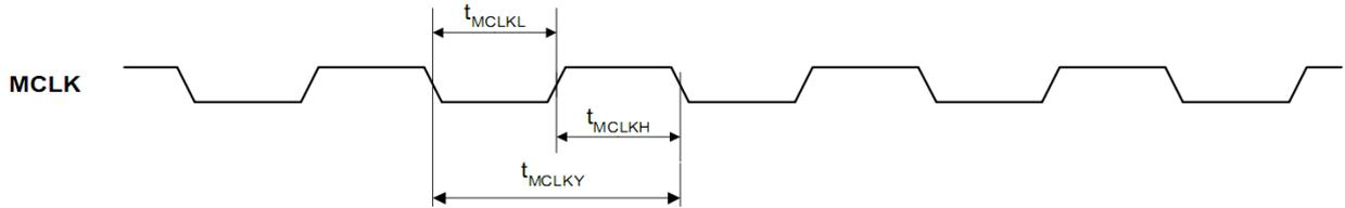
**Figure 1 System Clock Timing Requirements**
