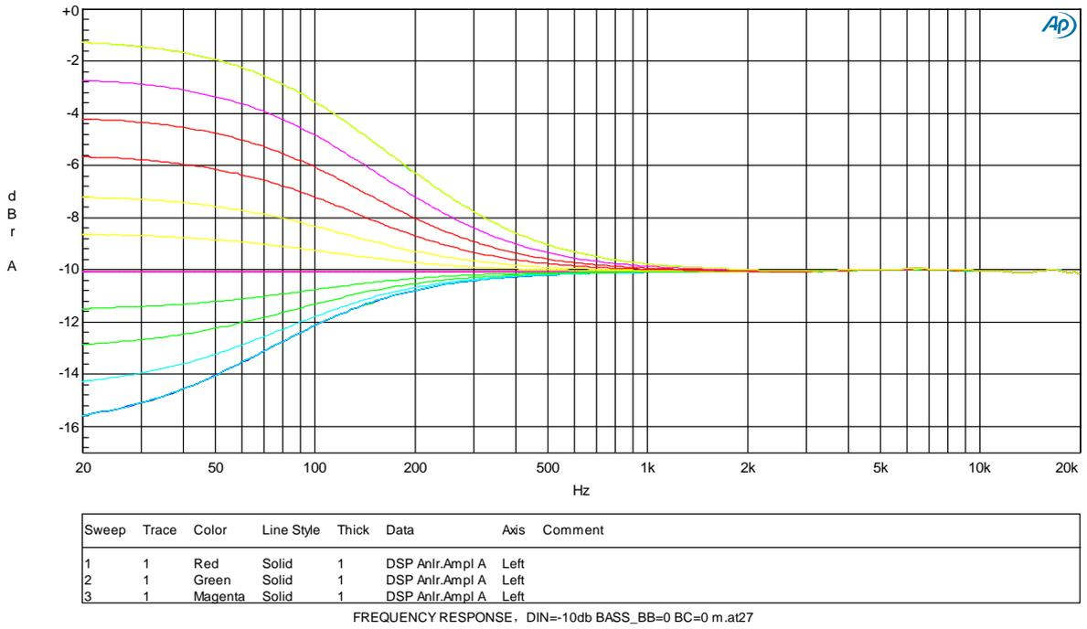
**Figure 32 FREQUENCY RESPONSE, DIN=-10db BASS\_BB=0 BC=0**
