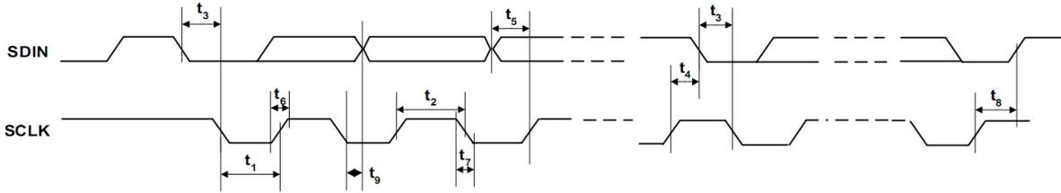
**Figure 5 Control Interface Timing – 2-Wire Serial Control Mode**
