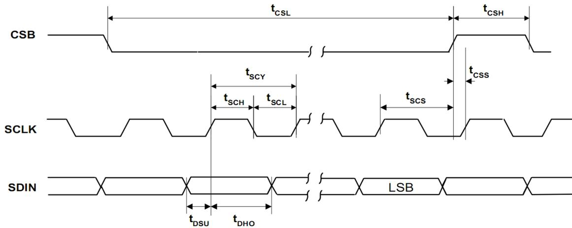
**Figure 4 Control Interface Timing – 3-Wire Serial Control Mode**
