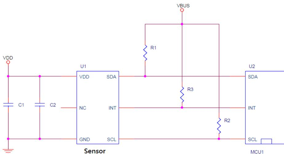
The capacitors (C1, C2) are required for power supply. The capacitors should be placed as close as possible to the device. The high frequency AC noises can be shunted to the ground by the capacitors. The transient current caused by digital circuit switching also can be handled by the capacitors. A typical value 0.1 / 1  $\mu$ F can be used.
