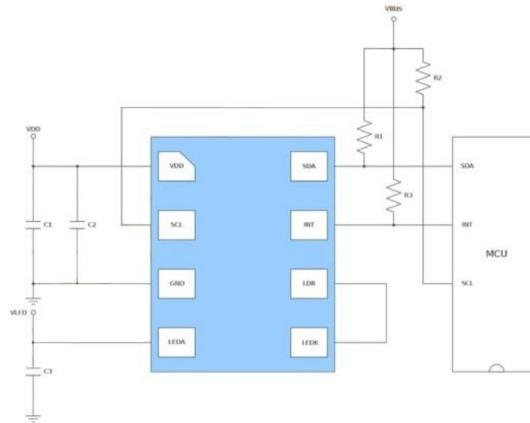
The capacitors (C1, C2) are required for sensor power supply. The capacitors should be placed as close as possible to the device. The high frequency AC noises can be shunted to the ground by the capacitors. The transient current caused by digital circuit switching also can be handled by the capacitors. A typical value 0.1 / 1  $\mu$ F can be used.
