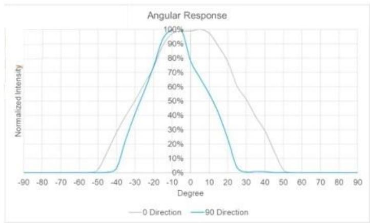
Fig. 5 IR LED Angular Response
